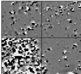
Magnetic debris consists of numerous dipolar responses spread over an area. If the amplitude of response is low ( $\pm 3\text{nT}$ ) then the origin is likely to represent general ground disturbance with no clear cause, it may be related to something as simple as an area of dug or mixed earth. A stronger anomaly ( $\pm 250\text{nT}$ ) is more indicative of a spread of ferrous debris. Moderately strong anomalies may be the result of a spread of thermoremanent material such as bricks or ash.
