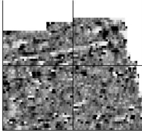
A linear response which is entirely negative in polarity. These are generally caused by earthen banks where material with a lower magnetic magnitude relative the background top soil is built up. See also ploughing activity.
