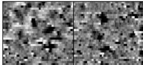
These are generally spatially small responses, perhaps covering just 3 or 4 reading nodes. They are entirely positive in polarity. Similar to positive linear anomalies they are generally caused by infilled cut features. These include pits of an archaeological origin, possible tree bowls or other naturally occurring depressions in the ground.
